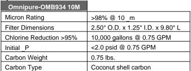
Notes: Chlorine reduction capacity based on laboratory testing conducted using test protocol contained in NSF Standard 42.
