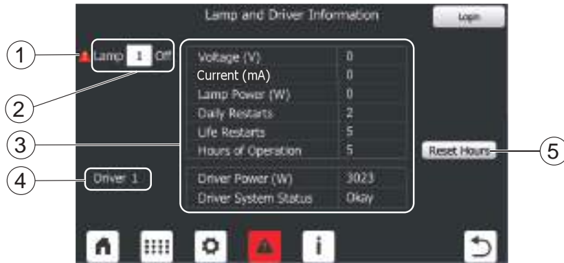
Figure 4 Lamp and Driver Information Screen - Active Lamp Fault Condition
