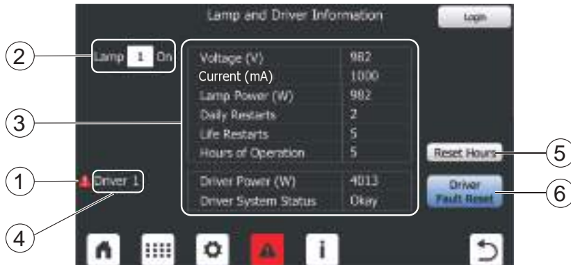
Figure 5 Lamp and Driver Information Screen - Active Lamp Driver Fault Condition
