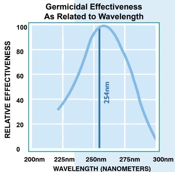
Approximately 95% of the ultraviolet energy emitted from **STER-L-RAY®** germicidal lamps is at the mercury resonance line of 254 nanometers, the region of germicidal effectiveness most destructive to bacteria, mold and virus.
